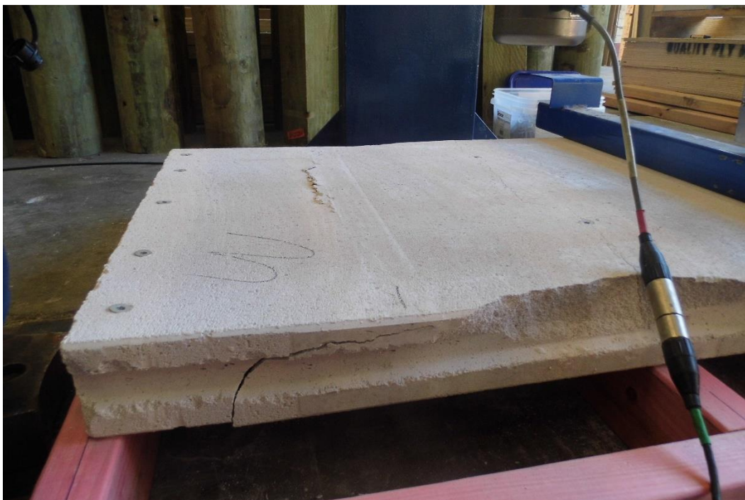
Figure 7 Flexural cracking and local compression crushing during uniform distributed load simulation testing
