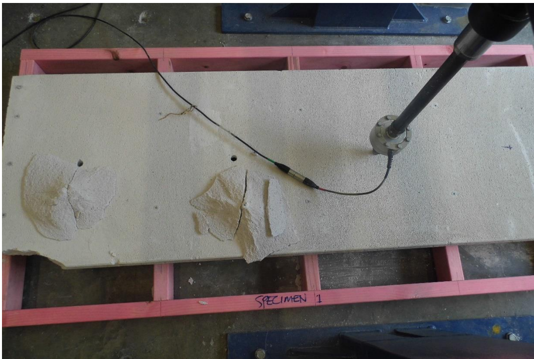
Figure 5 Concentrated load simulation tests underway
