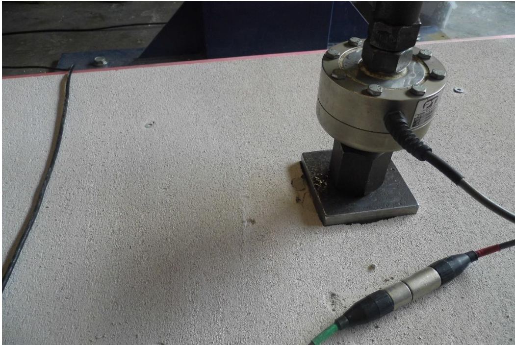
Figure 10 Typical local crushing of the top surface of the panel (100 mm x 100 mm foot)
