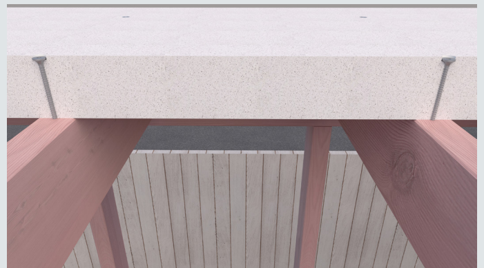
Image 5 – The ends of adjacent panels should finish over solid timber
