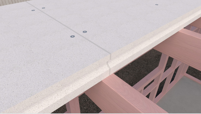
Image 5 – The ends of adjacent panels should finish over solid timber
