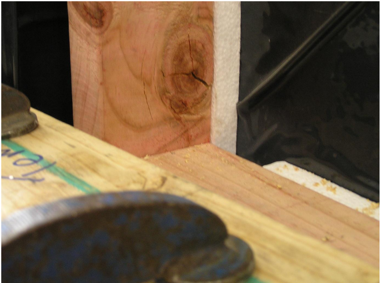
Figure 6. Stud cracking at a knot at 5.5 kPa and stiffening piece G-clamped to strong-back
