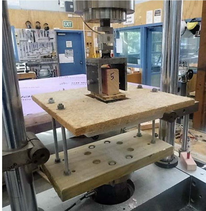
Figure 2. Typical Rockcote Pull-Off Specimen during Testing
