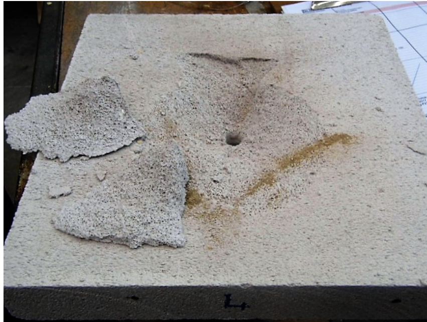
Figure 3. Typical Damage to Rockcote AAC Panels during Testing
