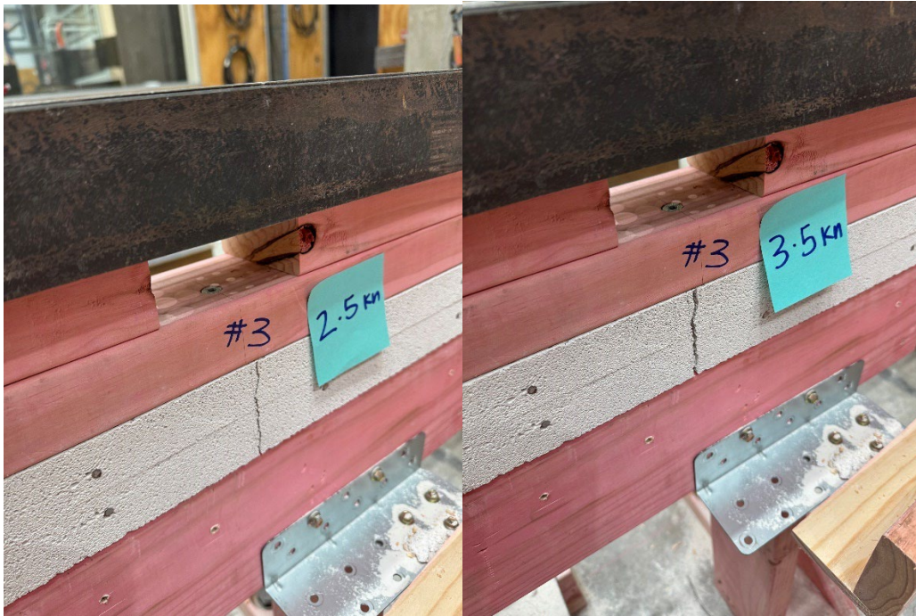
Figure 12 In plane testing: cracking of the flooring panel began on the 2.5 kN cycle
