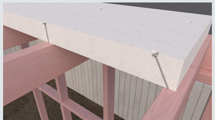
Image 8 – Skew fix the panel where the screws are located near the edge of the panels
