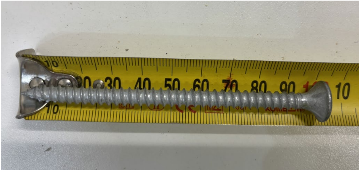
Figure 3 14g 100mm screw for fixing integra floor panel to joist.
