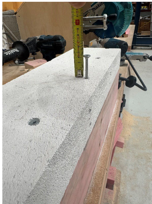
Figure 7 Tension test sample indicating 45mm of screw above floor plate.
