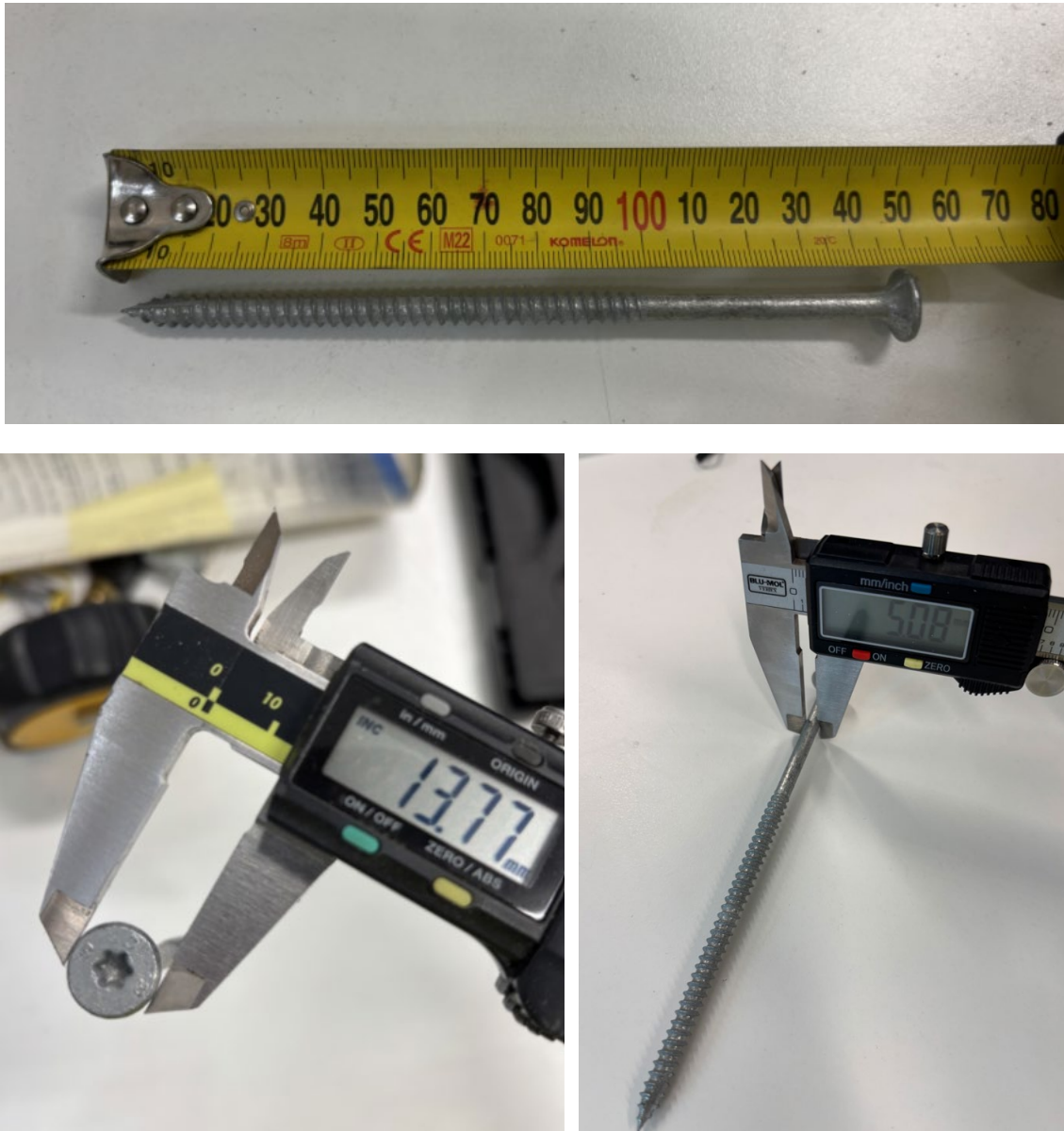
Figure 2 integra screw 150mm x 14g countersunk used to fix bottom plate.
