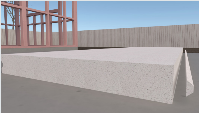
Image 2 - The tongue should be removed before installing the panels to the boundary joists
