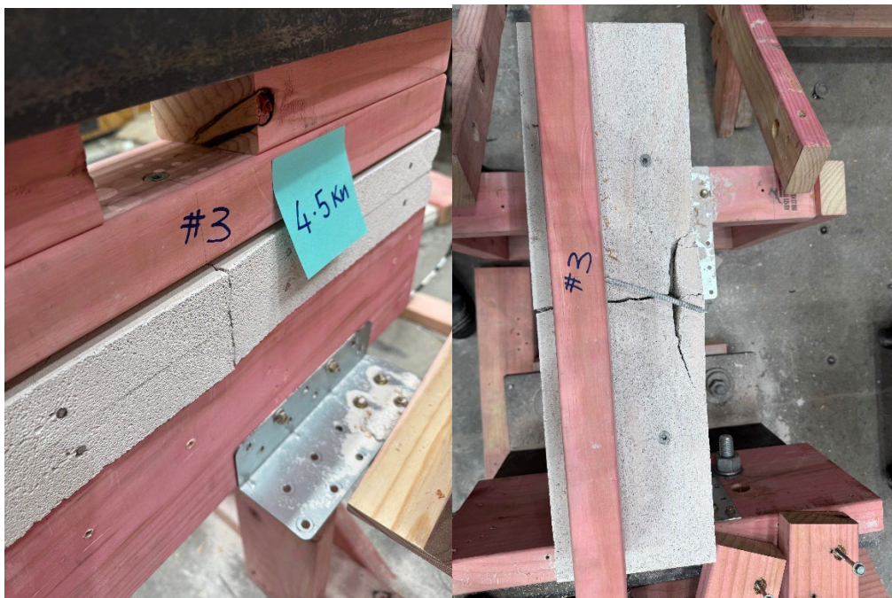
Figure 13 In plane failure of a sample (typical) where initial break out of floor panel is followed by pull out of the screw from the joist.
