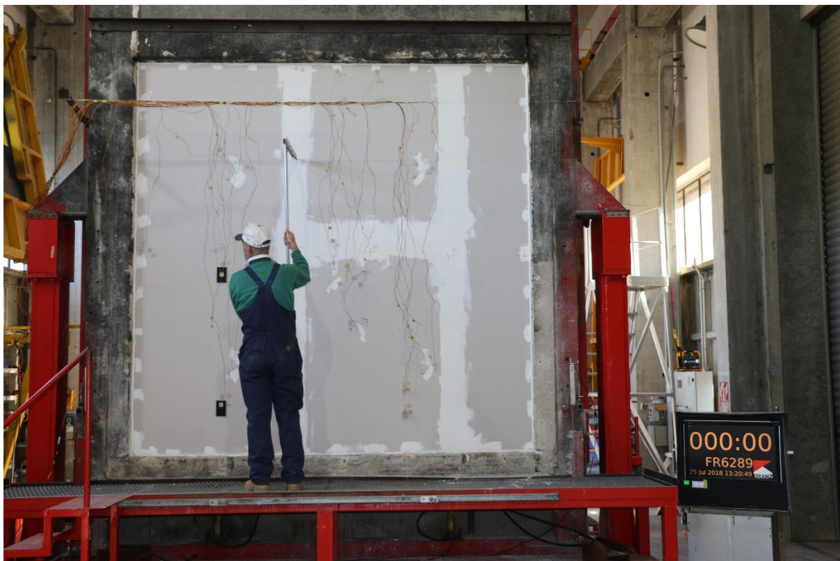
Photo 4: The Unexposed Face of the Wall After 125 Minutes
