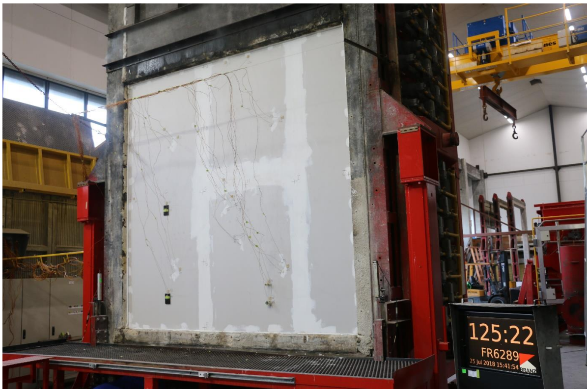
Photo 4: The Unexposed Face of the Wall After 125 Minutes
