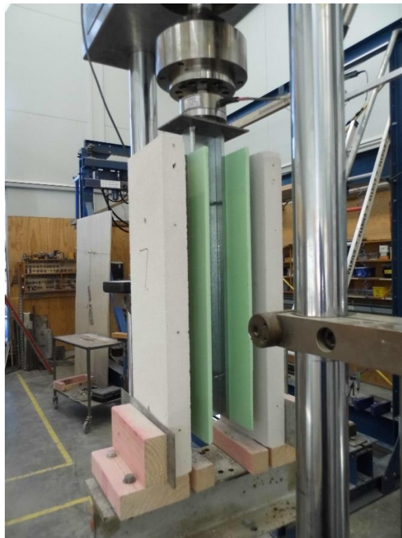
Figure 2. Sample Shear Test Specimen (Steel Stud)
