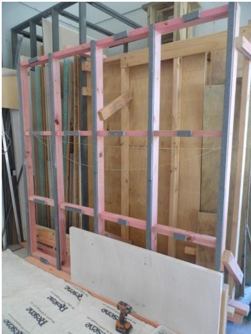
**Photo 2: Specimen with AAC panels installed**
