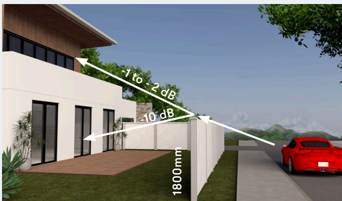
The reduction in noise with an Integra Fence in relation to a house.
