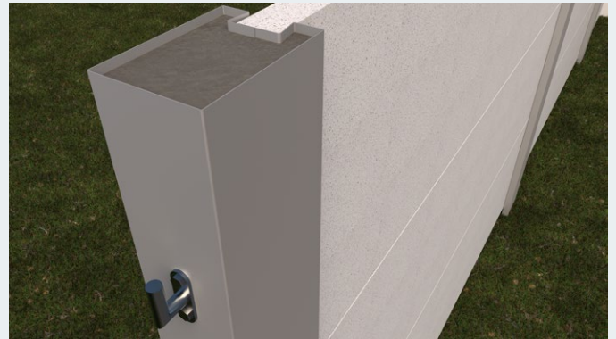
Gate fixings have been secured through into the concrete core.
